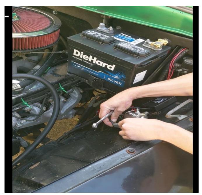
Install your stock ground cable terminal onto solenoid and tighten with 1/2" wrench.
