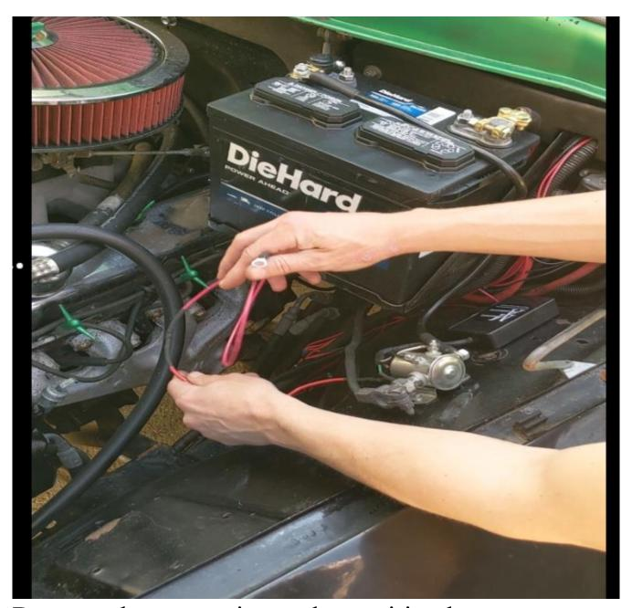
Route red power wire to the positive battery terminal and attach with 1/2" wrench.
