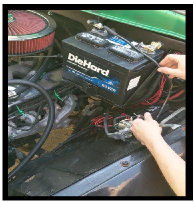
Bend new ground cable to achieve a desired shape from the solenoid to the battery, Install and tighten both ends of new ground cable and terminals.
