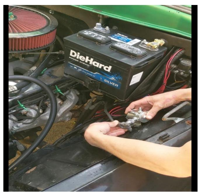
To start, Remove the negative ground terminal from your battery and check for the best mounting location of the solenoid. If you need longer ground cables, we have them available on our website; www.millstoneautomotive.com
