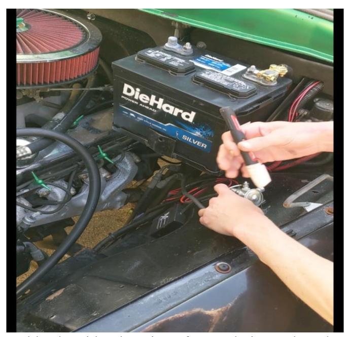
Hold solenoid to location of your choice and mark mounting hole with paint marker, Make sure you have room to drill pilot-holes without interference. Use 1/8" Drill bit and cordless drill to make pilotholes on marked location.
